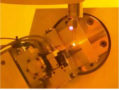
Laser sharpening generating no efforts on the tool, the mass and the kinetic of the machine have been developed specifically to ensure very fast and precise movements.
