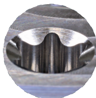
Machined Torx socket with REF 1450H
